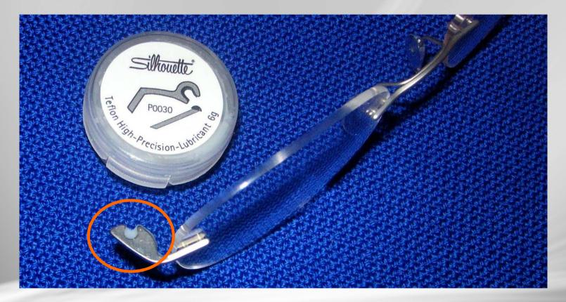
After cleaning grease inside loop of hinge with Teflon High-Precision-Lubricant P 0030. Afterwards mount temple.
